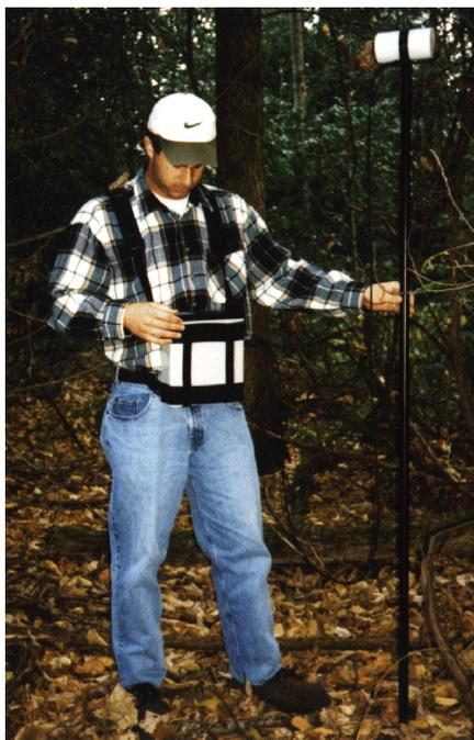
standard GEM capabilities: the Walking Mag option that enables the operator to sample while walking. Having nearly continuous data on survey lines also helps to increase the accuracy of interpretations.
