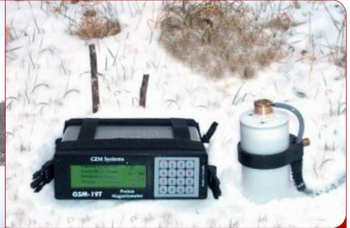
GSM-19TGW Proton Precession console configured with backpack, additional sensor for gradiometer (simultaneous) readings, built-in GPS and VLF EM system
